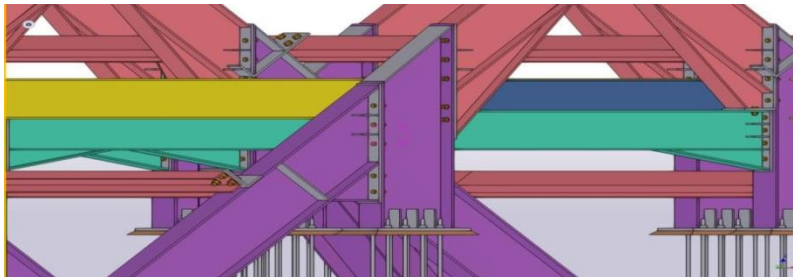
Gambar 8 Detail Sambungan Kuda-Kuda (Sumber: Tekla Structures )
